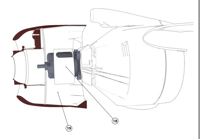
Attach the stabilizer (18) to the electric motor and screw the assembly to the nacelle and put the engine cover on the nacelle.
